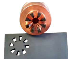
Electrode with ceramic mould
