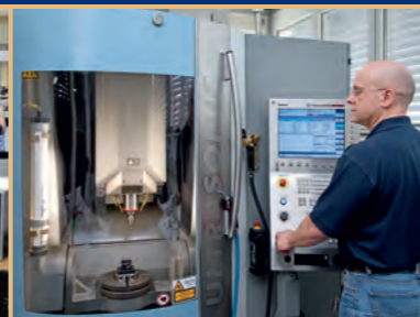
5-axis simultaneous milling is one of our core capabilities
