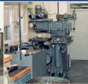
A profile milling machine dating back to the 1970s
